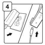
Plug in the power adaptor and connect the USB cable to the MimioTeach.
