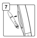
Rest the stylus in the cradle on the left of the MimioTeach bar. The stylus will begin to charge, and the ring will glow green when the stylus is ready.
