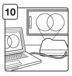
Calibrate the MimioTeach by pressing the calibration button  $(\oplus)$ .
