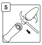
Unscrew the end of the MimioTeach stylus and remove the protective plastic strip to begin charging the batteries.
