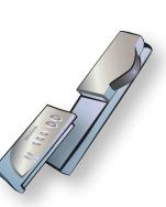
Insert/slide the Wireless Module into the mimio Xi.
