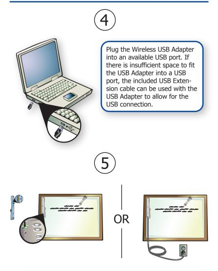
Power on mimio Xi. mimio Xi can be powered by 4 AA batteries or the included AC Adapter.
