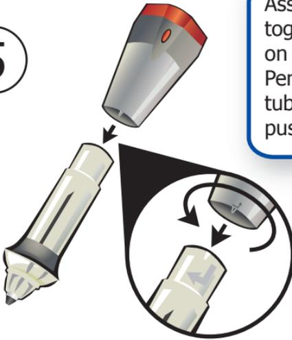
Assemble the Stylus Pen back together by aligning the arrow on the back end of the Stylus Pen with the arrow on the clear tube of the Stylus Pen and then push together and twist to lock.
