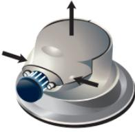
Remove the Eraser cover, by pressing on the sides of the Eraser and pulling.
