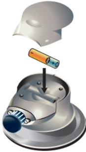
Insert AAA battery and assemble cover back onto Eraser.
