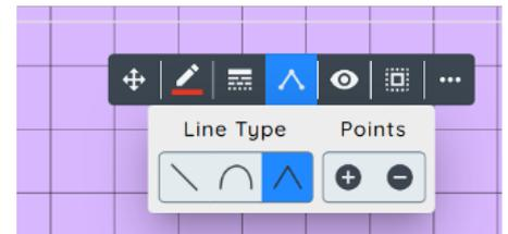
12 You can switch between the different line tools by selecting the line type and clicking on a different one.
