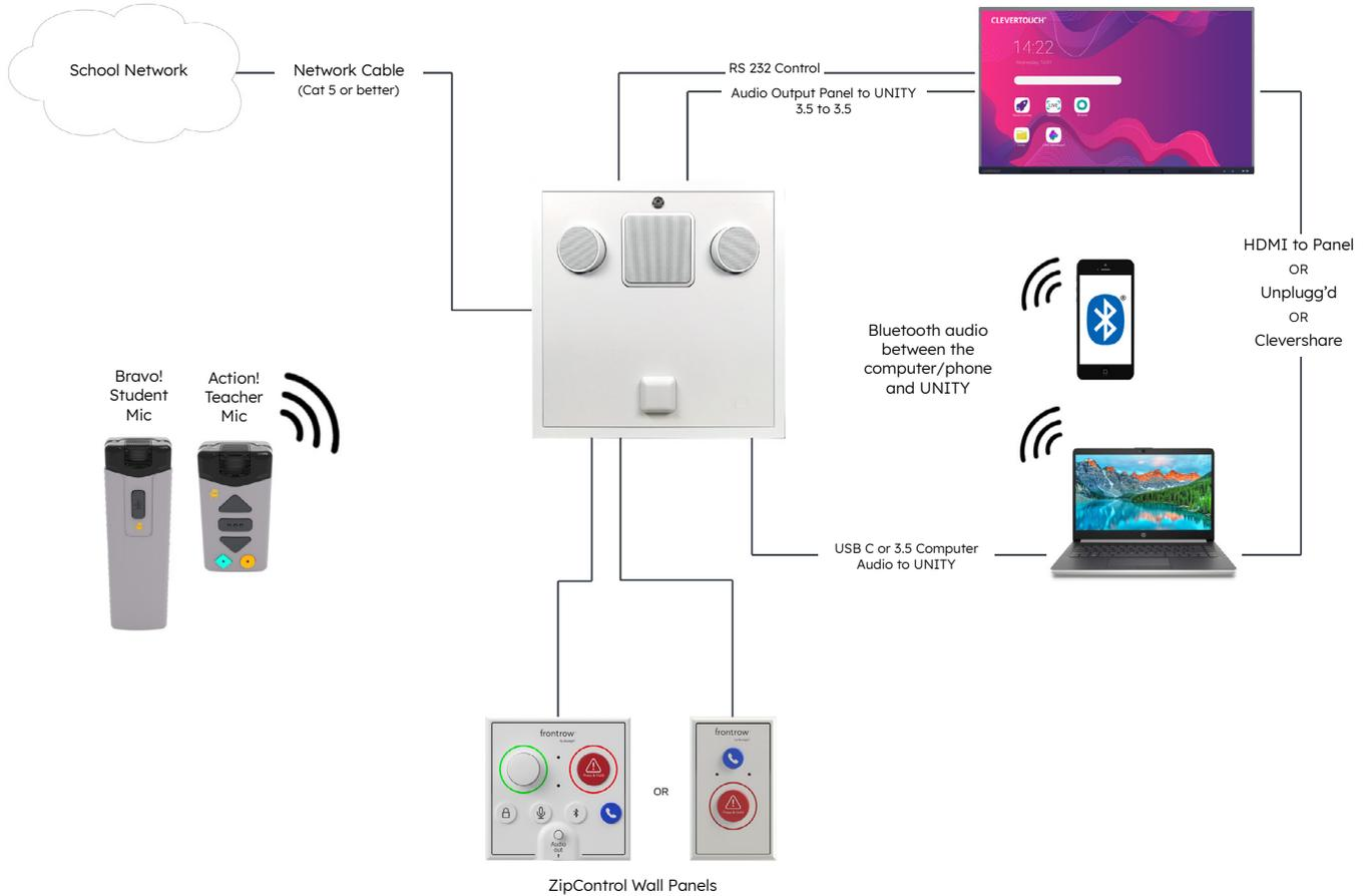
**NOTE:** When installing and turning Unity on, if connecting ClassLight make sure it is plugged in before power is supplied. ClassLight is not designed to be "hot-plugged" and unplugged.
