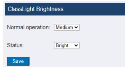
**Normal operation** pertains to general system changes. As an example; putting the Action microphone into Solo mode. The ClassLight will display Yellow with medium brightness.
