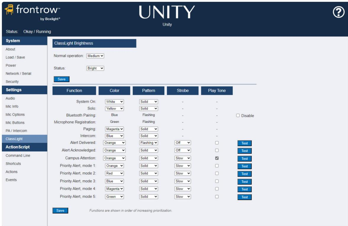
While ClassLight is customizable, the following information is based on UNITY's default settings when the ClassLight is installed.
